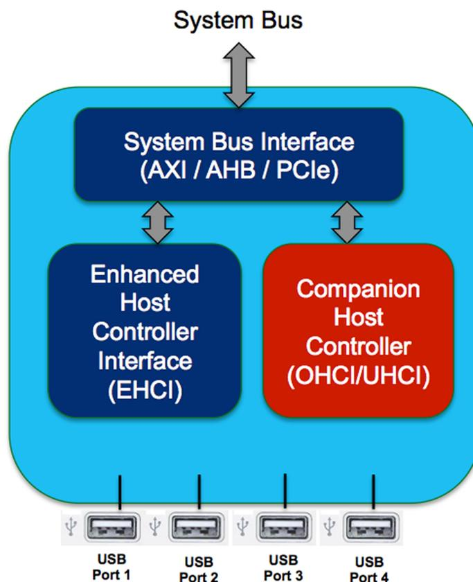
**Figure 2: USB 2.0 Host controller with companion host controller**
